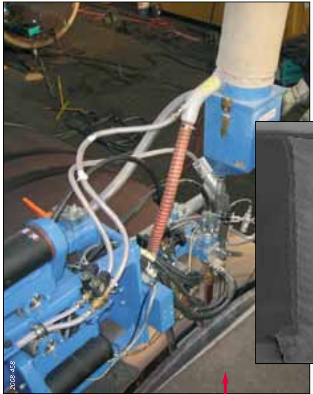
Single and tandem narrow gap up to 250 mm wall thickness
