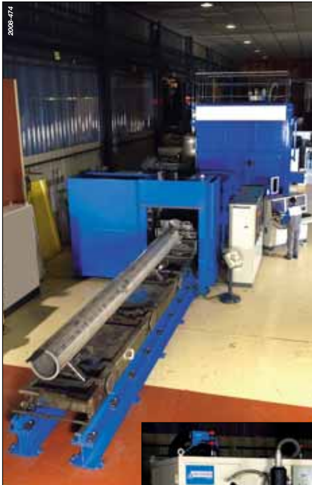
Machine for tube welding with gun inside the chamber.
